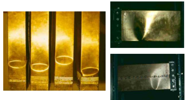
Fig. 62. At left different distances from fastened end of hinges (breaking point in lower part - dependently on boundary conditions) for thin-walled cantilevers (Fig. 59) and at right views from both sides.
